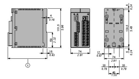
When using XPSMCTS• connectors this dimension is 153 mm (6.02 in)
