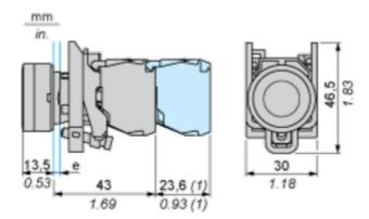
$\boldsymbol{e}$  : clamping thickness: 1 to 6 mm / 0.04 to 0.24 in. (1) Additional row of contacts or double contact
