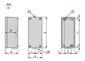
(1) 1 hole, without blanking plug, for cable gland with 18 mm/0.71 in. maximum clamping capacity
