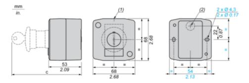
(1) 2 knock-outs for Pg 13.5 cable gland, maximum capacity 12 mm/0.47 in. (2) Knock-out for cable entry, maximum capacity 14 mm/0.55 in.
