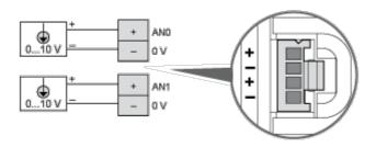
The (-) poles are connected internally.
