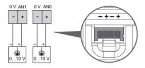
The (-) poles are connected internally.
