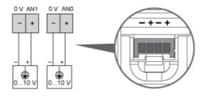
The (-) poles are connected internally.
