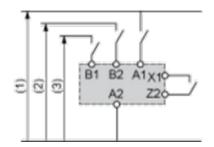
1 Supply 2 12...48 V 3 24 V **Connection of Potentiometer**
