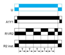
Before power-up Y1 should be permanently connected to A1. 2 timed outputs (R1/R2) or 1 timed output (R1) and 1 instantaneous output (R2 inst.)
