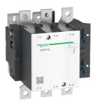
TeSys F contactor - 3P (3 NO) - AC-3 - <= 440 V 115 A - coil 200...208 V AC
