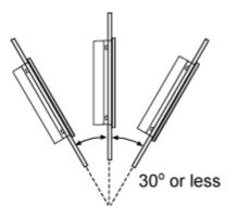
When installing the panel in a slanted position with an incline more than  $30^{\circ}$ , the ambient temperature must not exceed 40 °C (104 °F). You may need to use forced air cooling (fan,A/C) to ensure the ambient operating temperature is  $40^{\circ}$ C or less (104 °F or less).
