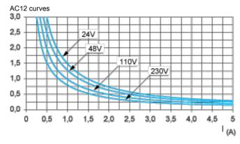
AC12 control of resistive loads and of solid state loads isolated by optocoupler,  $\cos \phi \ge 0.9$ .
