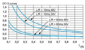
DC13 switching electromagnets,  $L/R \le 2 \times (Ue \times Ie)$  in ms, Ue: rated operational voltage, Ie: rated operational current (with a protective diode on the load, DC12 curves must be used with a coefficient of 0.9 applied to the number in millions of operating cycles)
