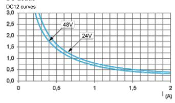
DC12 control of resistive loads and of solid state loads isolated by optocoupler,  $I/R \le 1$  ms.
