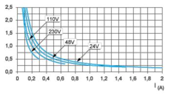
AC14 control of small electromagnetic loads  $\leq$  72 VA, make:  $\cos \varphi = 0.3$ , break:  $\cos \varphi = 0.3$ .
