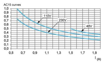
AC15 control of electromagnetic loads > 72 VA, make:  $\cos \phi$  = 0.7, break:  $\cos \phi$  = 0.4.
